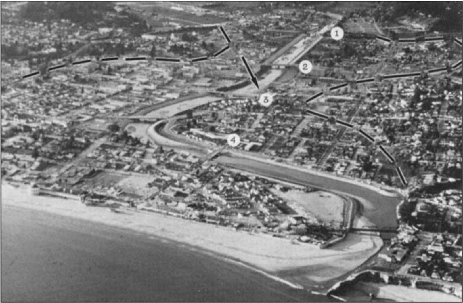
The city of Santa Cruz and the San Lorenzo River Flood Control Project in 1971. Dashed line delineates the floodplain. Numbers refer to individual bridges—1) Highway 1, 2) Water Street, 3) Soquel Avenue, 4) Riverside Avenue. Arrow indicates point where Branciforte Creek enters San Lorenzo River.
