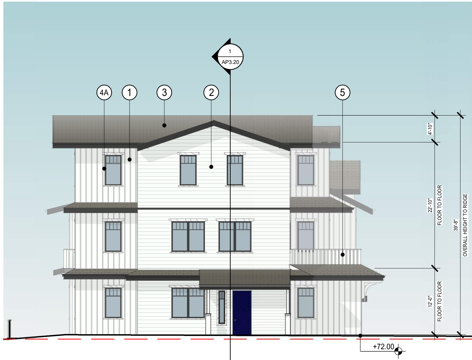
WEST ELEVATION - UNITS 1-5 3 3/32" = 1'-0"
