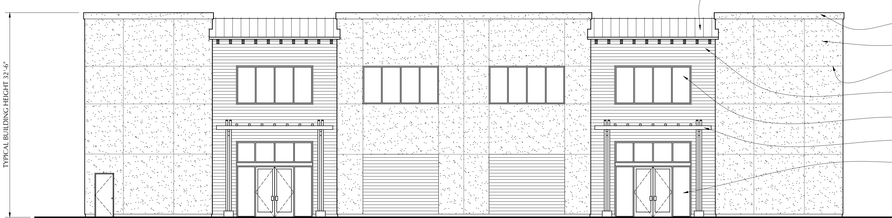
1 BUILDING 'A' SOUTH ELEVATION SCALE: 1/8"=1'-0"
