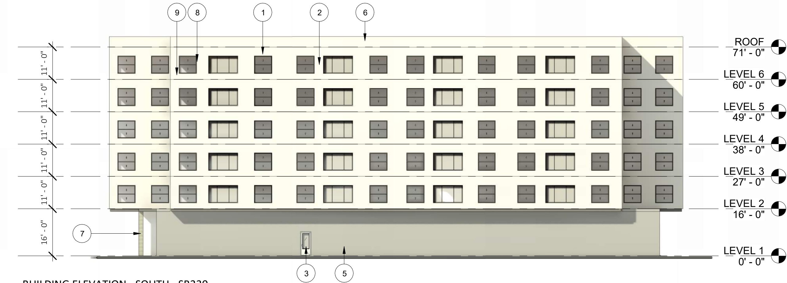
3 BUILDING ELEVATION - SOUTH - SB330 1" = 20'-0"
