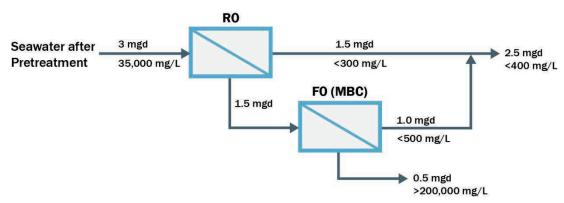
Figure 1. Water Balance Diagram with RO Brine Concentration by Forward Osmosis Membrane Brine Concentrator (MBC)
