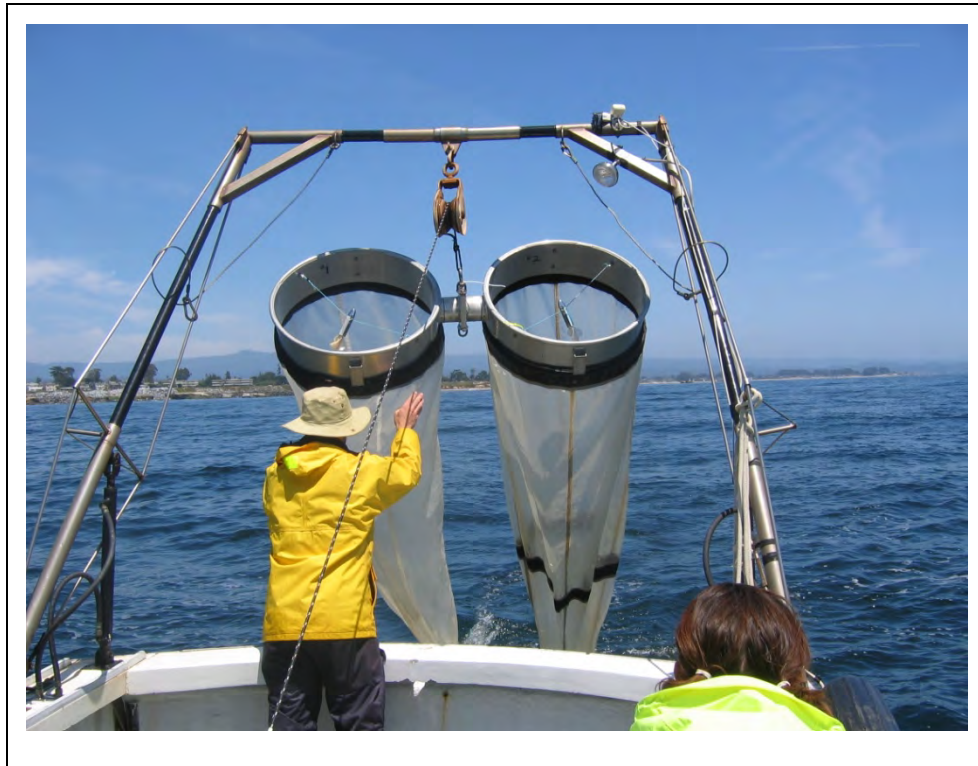
Figure 3.2-2. Bongo frame and plankton nets used to collect fish, shrimp and crab larvae at the proposed intake and in the source water.
