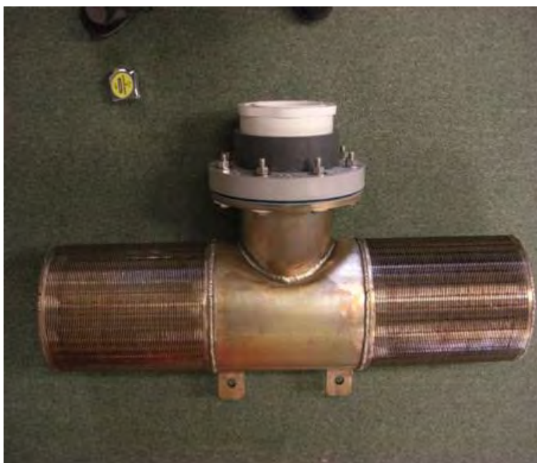
Figure ES-2. Pilot-scale narrow-slot wedgewire intake screen.
