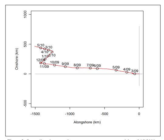
**Figure 2**. Coast-aligned water column average currents measured from 2/13/2009 to 5/13/2010 at a current meter located at Terrace Point maintained by the University of California, Santa Cruz, showing current displacement in a progressive vector. Movement was generally upcoast in the alongshore direction. From Tenera (2010).
